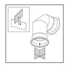
Place the stove pipe on top of the stove and push the stove pipe against the wall/back panel.
